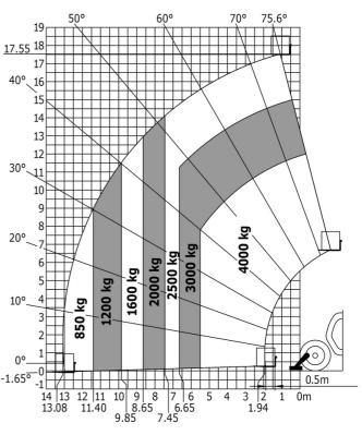
Machine on stabilisers with Man basket Metric
