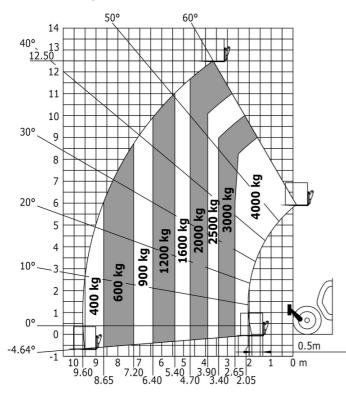
Machine on lowered stabilisers with forks Metric
